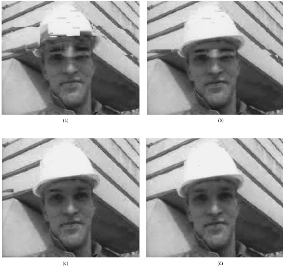
Fig. 19. Reconstructed frames of test sequence Foreman : (a) frame 90 after previous frame concealment of two GOB's in frame 75; (b) as (a) with INTRA update in frame 90 according to Same GOB strategy; (c) as (a) with INTRA update in frame 90 according to error tracking strategy; (d) frame 90 without GOB loss in frame 75.
